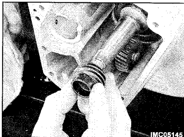
Figure 349 — Removing spacer and oil pump drive gear
